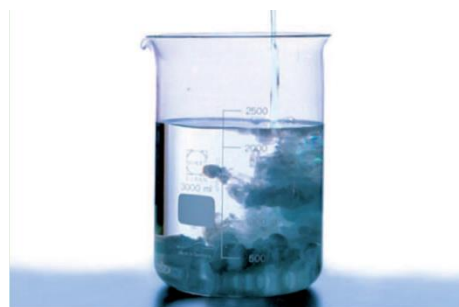
Picture 1: Blooming effect of a self-emulsifying oil with IMWITOR® PG3 C10
